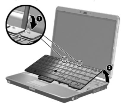
6. Holding the keyboard at an angle, lift the keyboard (1) far enough to gain access to the cables underneath and release the zero insertion force (ZIF) connector (2) to which the pointing stick cable is attached to the system board and remove the pointing stick ZIF cable (3) from the connector.
